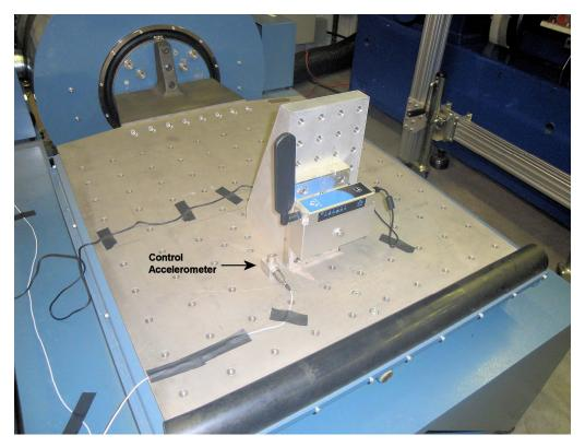
Figure 1.2.1 Y Axis Setup (Control from Slip Table)
