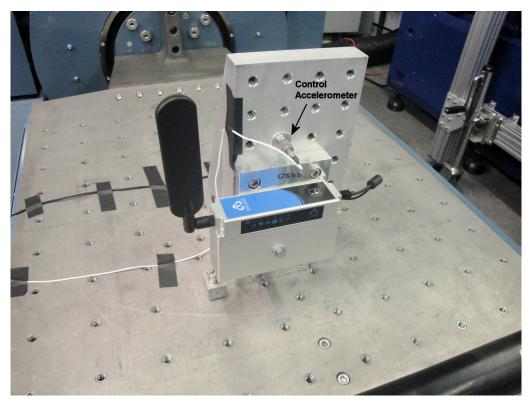
Figure 1.2.2 Y Axis Setup (Control from Angle)
